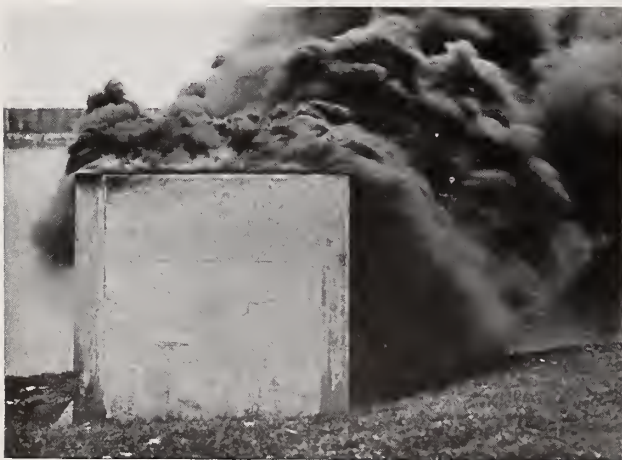
Terrific heat of 160 gallons of burning kerosene has no effect on Hy-Rib Concrete Tank. Size: 5' x 5' x 5', 3 ins. thick.
