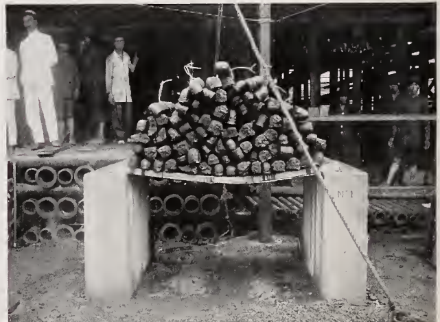
2 in. Concrete Slab reinforced with Hy-Rib. 5' 3/4" clear span. Designed for 112 lbs. per sq. ft. Load carried 625 lbs. per sq. ft.
